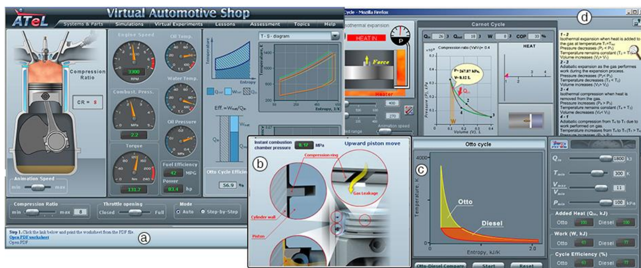
Figure 4. The virtual experiment “Influence of Compression Ratio on Engine Operation Cycle” performed at the v-Lab “Internal Combustion Engine Design and Operation”
